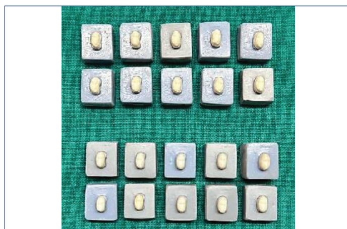
[Table/Fig-1]: Resin dies fabricated from 3D printer.
